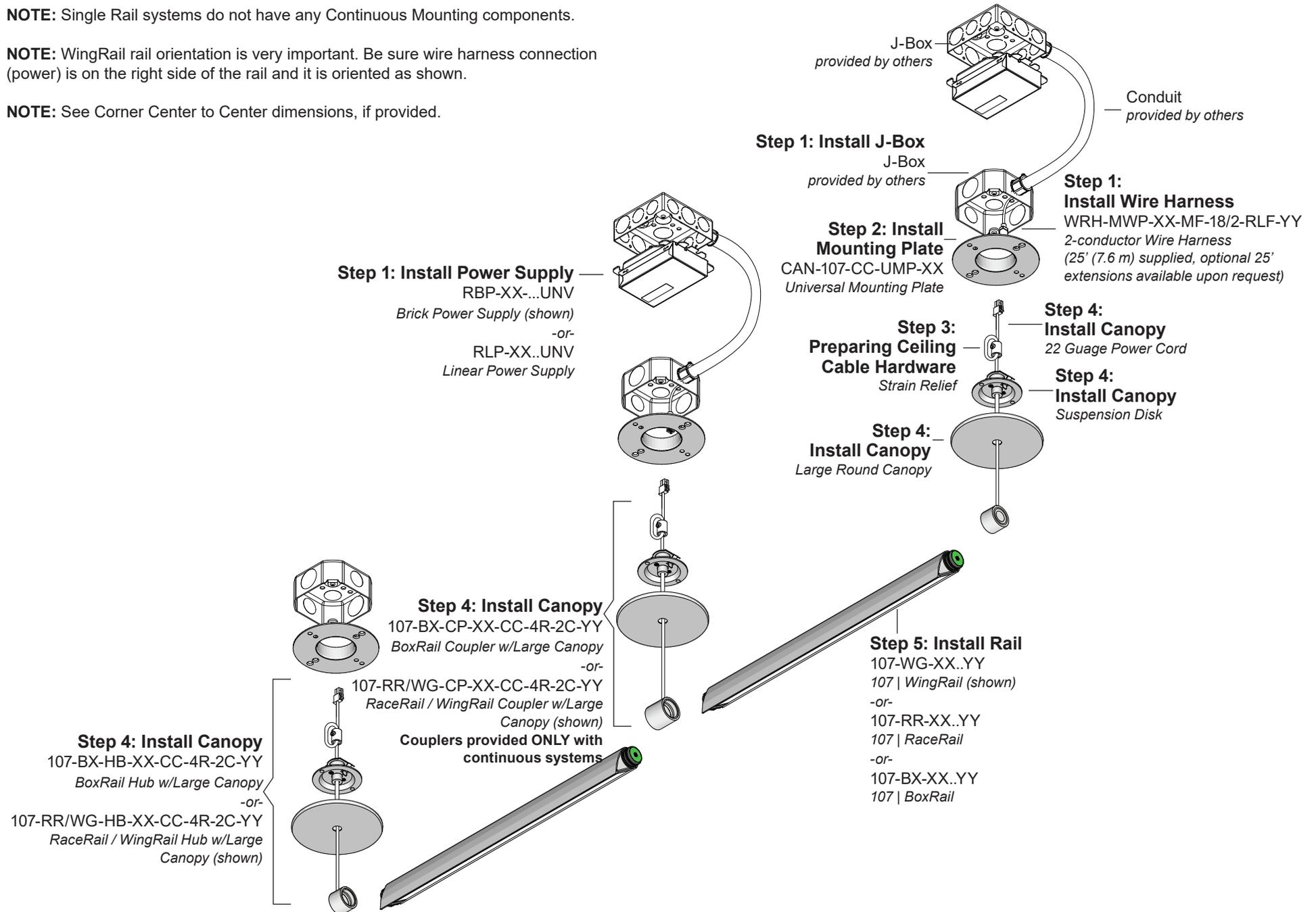
**Step 1: Install J-Box, Power Supply and Wire Harness**
