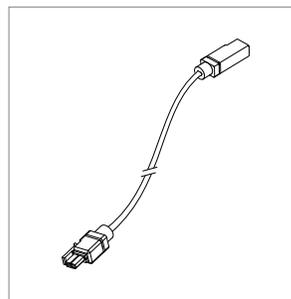
Wire harness connects driver to rail. Wire harness is 25' (7.6m) with micro fit molex connectors for quick and easy installation. Multiple harnesses can be combined for a total length of up to 100' (30.5m). See [Tech Sheet](#) for details.
