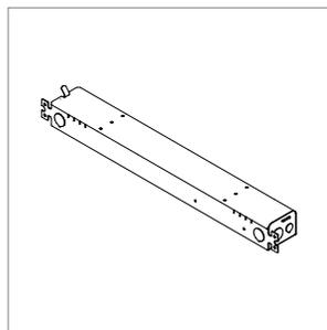
One remote power supply housing is supplied with each power supply. All Vode linear remote drivers come in a 0.054" (0.8mm) formed galvanized steel power supply housing with five (5) knockouts: (4) 1-1/8", (1) 7/8" and (1) 9/16". Accommodates standard linear power supplies. See [Tech Sheet](#) for details.
